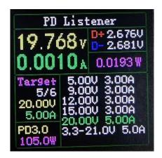
In the figure above, the charger is a 105W PD charging head. The current PD consumer selects the 5th gear and triggers the target voltage of 20V, the maximum current is 5A.
