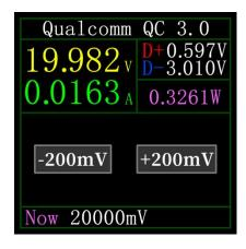
In QC3.0 trigger mode, use the left and right keys to decrease/increase the trigger voltage, and long press the OK key to return.
