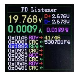
Click the middle button to switch to the "View Detailed Communication Process" page, as shown in the figure above.
